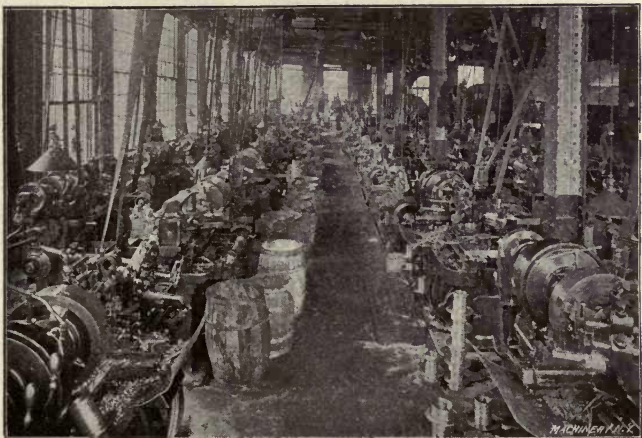
Fig. 28. An Unusual Array of Automatic Chucking Machines; Thirty-one are used in this Department
